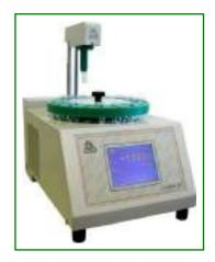
Code no. 67165 40-sample double-headed cryoscope – CryoStyle 40 Double
